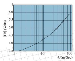
This graph is made for the "Top ofthe bridge" voltage with no signal conditioning.
