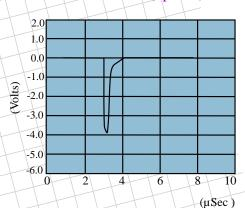
Impulse input: 4 V amplitude, 400 nsec width
